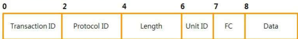
MODBUS TCP Frame Structure
