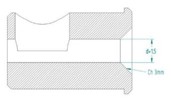
Choice C: Solid bit holder machined according to the following drawing
