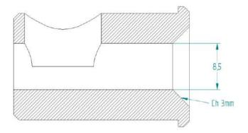
Choice B et D: Solid bit holder machined according to the following drawing
