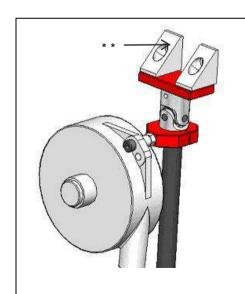
Attach the arm as shown in the image. Take care to orient the cardan for the required work area.
