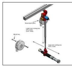
Attach the arm as shown in the image. Take care to orient the pivot for the required work area.
