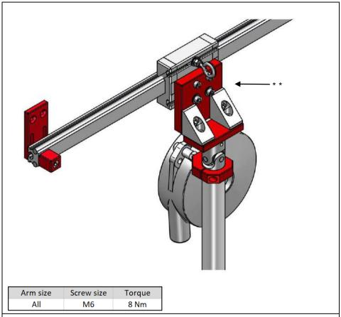
Attach the arm on the rail as shown in the image.
