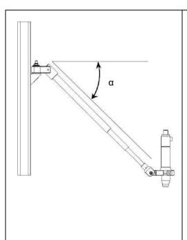
It is imperative to respect the angles indicated below in the working position while installing the DMF arm.
