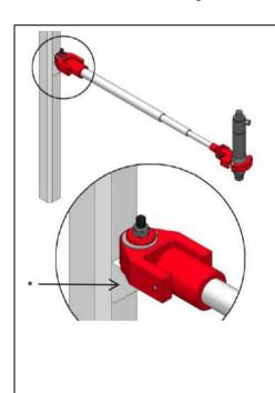
Attach the arm to a post as shown in the image. Take care to orient the pivot for the required work area.
