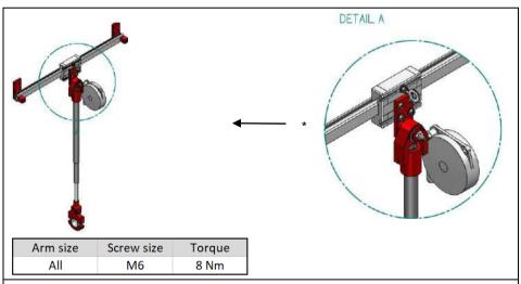
Attach the arm on the rail as shown in the image.
