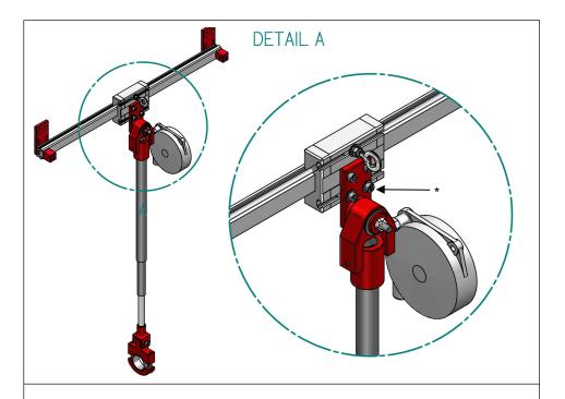
Attach the arm on the rail as shown in the image.
