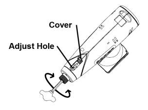
2. Use the torque adjust tool to turn clockwise to increase torque and turn counterclockwise to decrease torque.
