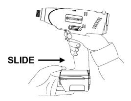
2. To remove the battery pack, press the red button on the top of the battery pack and release the battery pack.
